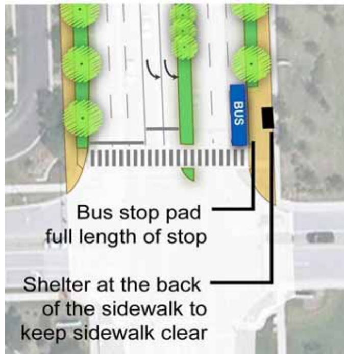
Concept sketch showing the typical preferred location of a far side bus stop on La Grange Road.
